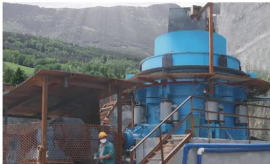
H series Hydraulic Multi-Cylinder Cone Crusher is world advanced level cone crusher, based on years of experience and world advanced technology, which can be widely used on metallurgy, construction, hydro-electric, transportation, chemical and construction material etc. It is always used to crush stones or ores of medium and high hardness.
